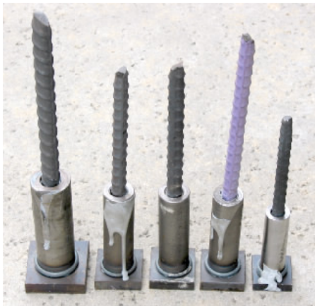
The epoxy-grouted connection consistently exceeds the actual stress and strain capacity of A706 rebar.
